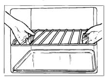
To position the DOUBLE DUTY™ shelf, tip the back slightly and fit the shelf support guides onto the support guides located on each side of the oven in the rear.
